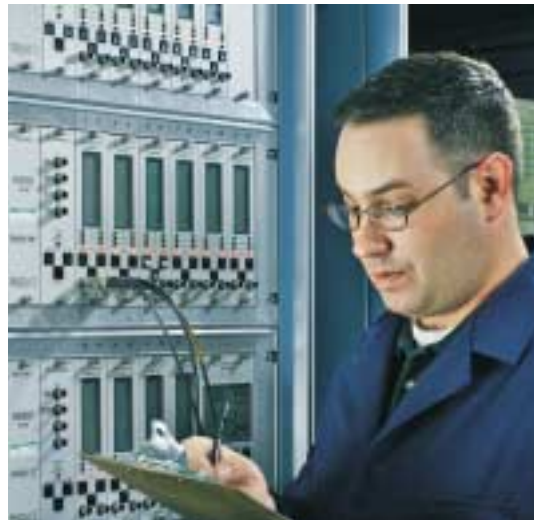
Cooper Compression's test center control room provides computer control of cooling water, input speed and lubricating oil supply.
