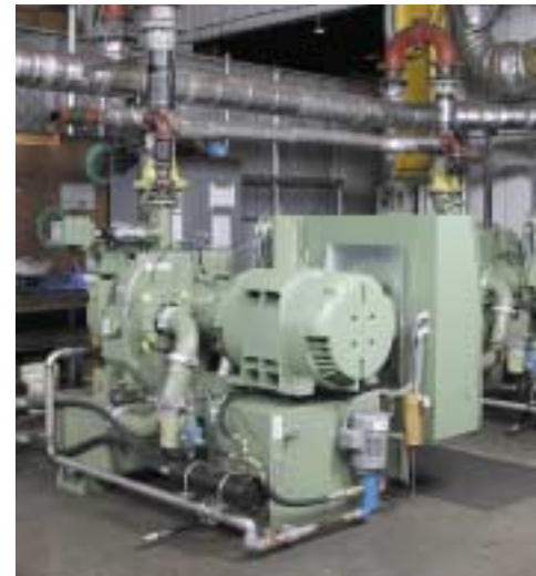
Standard package test of Turbo Air® 2000 in Cooper Compression test center.
